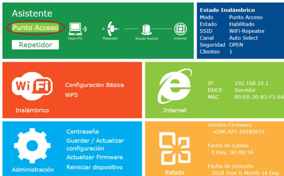
The screenshot displays a configuration interface for a WiFi Repeater. At the top left, a green 'Asistente' (Assistant) panel shows a diagram of the connection: User-PC connected to a Repeater, which is connected to a Router Switch, which is connected to the Internet. The 'Punto de Acceso' (Access Point) option is highlighted with a red circle. Below this, a blue panel shows the 'Estado Inalámbrico' (Wireless Status) with the following settings:
